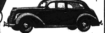
STANDARD FORD V-8 ... 112" wheelbase; 65 or 85 horsepower engine; Improved Easy-Action Safety Brakes; Center-Pole Ride; All-steel body; Broadcloth or Mohair upholstery; Mohair extra in '60"; Mahogany-finished trim; One tall light, sun visor; Twin horns; 3 body types; 3 colors.
